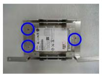
Step 6: Plug into HDD cable and you've done HDD installation
